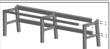
Align Left and Right Leg Assemblies with Aprons and Lower Rear Stretcher. Secure using (10) 50mm Hex Lags into pilot holes. Plug Holes with 5/8" taps® using a Rubber Mallet.
