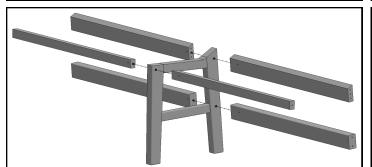
Align the angles on Left and Right Rear Aprons, with the hanger bolts towards center, to the Angle on rear of Center Leg Assembly. Thread in Aprons and Lower Rear Stretchers until tight and aligned as shown. ATTACH OUTER LEGS
