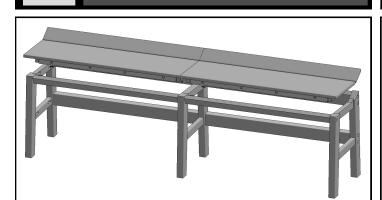
Rotate Front Apron slightly outward. Insert Seat Assembly, starting with the rear, and lightly tap until Seat "pops" in.
