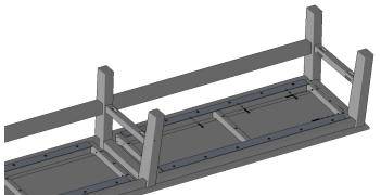
Hold Seat tight to Frame. For 216, hold Seats so slats are tight together in the center. Secure using (12) 1-1/4" Phillips Head Screws for 215, and (20) for 216.
