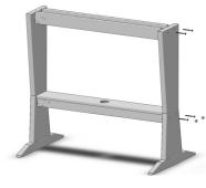
Attach Upper Stretchers and Stretcher Assembly to Leg Assemblies using (8) 80mm Hex
