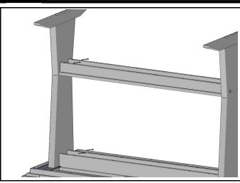
Secure Upper and Lower Stretchers using (8) 1-3/4" Phillips Head Screws through pockets in bottom of Stretchers into Legs.
