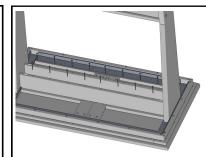
Attach Upper Stretchers to Table top using (16) 1-3/4" Phillips Head Screws.
