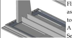
Flip over Base assembly on to Table Top Assembly. Secure Alumi-
