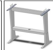
Align predrilled holes in Legs with holes in Aluminum Support Braces as shown. Secure using (6) 50mm Hex Lags.
