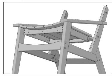
Drop Seat Assembly in between Aprons. Secure with (7) 1-1/4" Screws through counter-sunk holes in bottom of Seat, starting with holes in the front.
