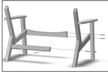
Align Front and Rear Aprons with Front and Rear Legs. Secure with (6) 50mm Hex Lags through counterbored holes in Legs, and (2) 1-3/4" Screws through pockets in Rear Apron. Plug holes in Legs with 5/8" taps®.
