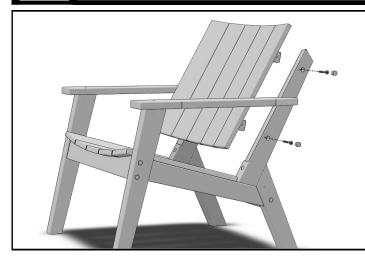
Align pilot holes in rear stretchers of Back Assembly with the counterbored holes in the Rear Legs. Secure with (4) 50mm Hex lags. Plug holes with 5/8" taps®.
