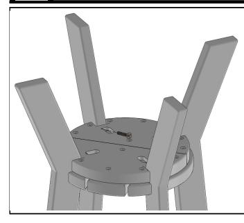
Secure Lower Shelf to Legs using (4) 1-3/4" Phillips Head Screws thru holes in shelf into legs.
