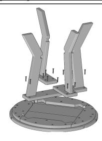
Align Legs to table top as shown with the angles pointing outward, and notches facing inward. Secure using (16) 1-1/4" Phillips Head Screws.
