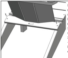
Place Back Assembly on top of mounting surface of Rear Legs (Part of Seat Assembly). Push Back Assembly forward until it meets the last Seat Slat of the Seat Assembly. Hold Back Assembly in place and install (2) 1-3/4" Phillips Head Screws into predrilled holes on each side of the Lower Yoke (No pre-drilled holes on Rear Legs).
