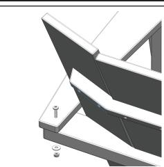
Place Upper Yoke of the Back Assembly underneath arms, aligning pre-drilled holes. Install (1) 60mm connector bolt through pre-drilled hole of the Arm and through Upper Yoke. Finger tighten flat washer and Lock Nut. Do not fully tighten at this time. Repeat process for opposite Arm.
