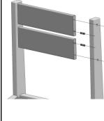
Tap 5/16" dowels into large holes in back slats. Align with large holes in rear legs. Secure with 1-3/4" Phillips head screws through 3/8" counterbore in Rear Legs into pilot holes in back slats.
