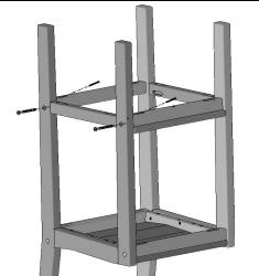
Attach Foot Rest and Rear Stretcher as shown, with pockets of Stretchers facing down, using (4) 80mm Hex Lags through counter-bored holes in Legs. Align straight, then secure using (4) 1-3/4" screws through pockets on underside of Foot Rest and Rear Stretcher.
