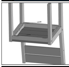
At this time make sure lags from step 2 are tight. Rotate rear apron to align with angle on seat support, and make sure front apron is parallel with front leg. Secure aprons with 1-3/4" Philips head screws through the pockets on underside of aprons into legs.
