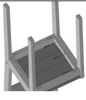
Align seat assembly with frame. Secure using 1-3/4" Philips head screws through countersink holes on inside of seat assembly into pilot holes in side assemblies.
