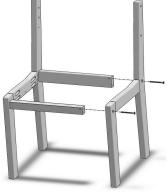
Attach front and rear aprons to Side Assemblies as shown, with the pockets of the aprons facing down using (4) 80mm Hex Lags through counter-bored holes in Legs.
