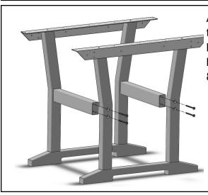
Attach Stretchers to legs through counter-bored holes in legs into pilot holes in stretchers using 80mm hex lags.
