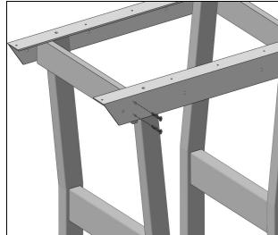
Attach short aprons to aluminum using 1-3/4" phillips head deck screws through holes in aluminum into pilot holes in short aprons.
