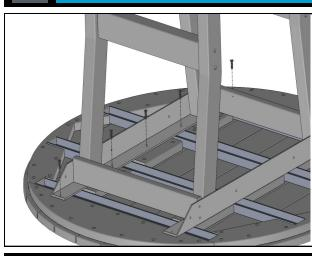
Align aluminum from base assembly with cleats on table top assembly. Secure using 3/4" pan head screws through holes in aluminum.
