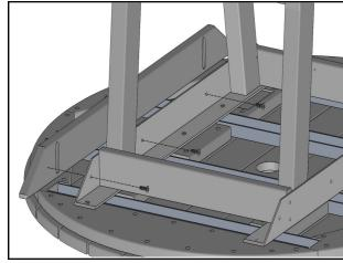
Align pockets in long aprons with protruding screw heads from step 3. Secure using 3/4" pan head screws.
