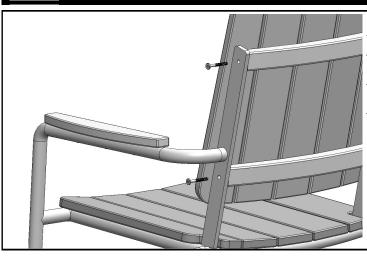
Align pilot holes in rear yokes of Back with the holes in the Chair frame. Secure with (4) 50mm Hex lags. Do not over tighten.
