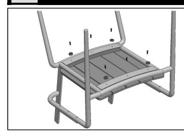
On a clean flat surface push seat tight to the front of the chair frame. Attach Seat with (6) 3/4" Phillips pan head screws. Secure Bumpers in locations shown. Do not over tighten.
