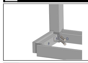
On a clean flat surface connect Legs to Frame Assembly with (2) 80mm Lags Per Leg (AS SHOWN). Do Not Over Tighten.
