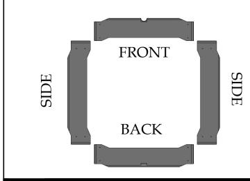
Begin by arranging parts on a flat surface as shown. Holes facing up. Take note of location of components.
