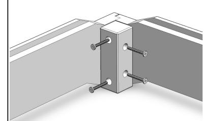
Using (16) 50mm Lags, align (4) CORNER with pre-drilled holes on FRONT, BACK, and SIDE(s). Do not tighten completely. Once (4) corners are upright and in position, fully tighten all hardware.
