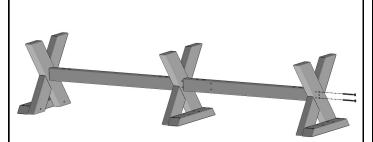
Align middle leg with mid cleat on Seat. Center the outer legs and secure using (24) 1-3/4" Phillips Head Screws.
