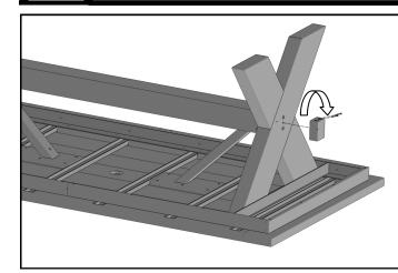
Align angle braces to stretcher assembly and table top as shown. Secure using (4) 1-3/4" Phillips Head Screws.
