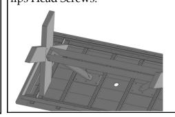
Insert End Caps into threaded insert in Leg Assembly. Turn clockwise until snug. Continue turning until in line with the Stretcher as shown. Secure end caps into legs with (4) 1-3/4'' Phillips Head Screws.
