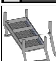
If you are assembling a Sofa (090), Align Mid Rear Leg with Rear Apron and Last Slat and Secure using (2) 2-1/2" Pan Head Screws thru holes in Rear Apron using a #3 Phillips Head Screwdriver.
