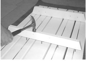
Place End and Center Cleat to Table Slat Carriage Bolts by taping them into place on all Carriage Bolts with a hammer and align cleats with numbers on slats. Attach Cleats using flat washers, nuts and finger tighten (Left Picture). Do not tighten at this time.
