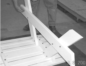
Place Seat Support along inside of legs, while aligning pre-drilled holes. Holes in Seat Supports must align with holes in the Table center Cleat for aligning and attaching the Angle Braces. Attach using (4) 3-1/2" Truss 5/16" Bolts. Finger tighten using flat washers and nuts (Left Picture). Do not tighten at this time. Repeat process on other side.
