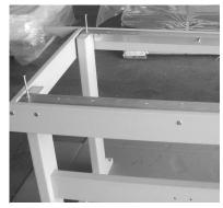
Place Apron Assembly on to Leg Assembly aligning pre-drilled holes in the Aluminum and Legs (Left Picture). Attach using (4) 3" Hex 1/4" Lags (Right Picture).
