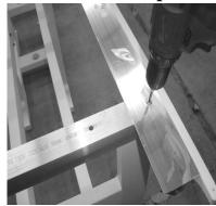
Place Aluminum Supports Brackets on the top of Outer Leg Assemblies aligning predrilled holes. Place Long Aprons across Outer Leg Assemblies and there Aluminum Support Brackets aligning all pre-drilled holes. Attach using (4) 3" Hex 1/4" Lags through Long Apron and Brackets. (Left & Right Picture)
