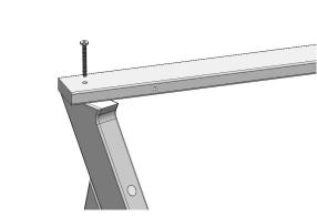
Attach Connector to legs using (4) 50mm Lags.
