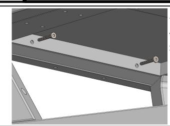
Attach Leg Assembly to Top using (4) 50mm Lags to Connector through aluminum holes.
