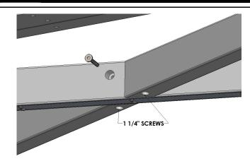
Attach Long Leg to Short Leg using (2) 50mm Lags and (2) 1 1/4" Philips head screws. Plug holes with 5/8" taps®.
