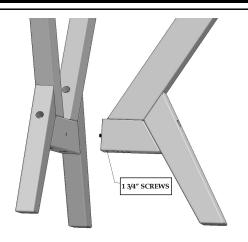
Screw Short Legs into Long Leg and secure from underneath using (2) 1 3/4'' Philips head screws.
