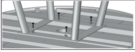
On a clean flat surface connect legs to top using (4) M6 Shoulder Screws, (4) M6 Lock Washers & (4) 1/4-20 Flat Washers (AS SHOWN). Do Not Over Tighten.
