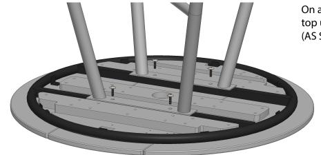
On a clean flat surface connect legs to top using (4) 316-1/4-20PPMS Screws (AS SHOWN). Do Not Over Tighten.
