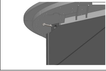
Drop Top onto Base and Secure using (4) 50mm Lags. Plug holes with 5/8'' taps®.
